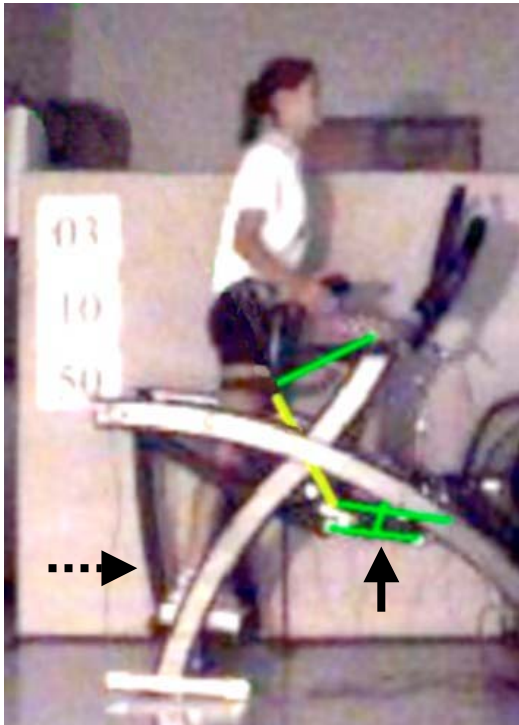
Figure 12. Parallelogram and foot plate of the arcuate cross trainer.
